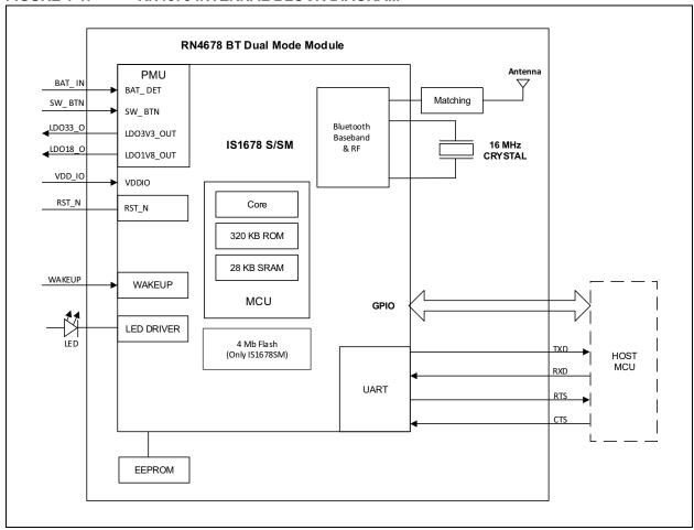
Table 1-1 provides the description of the various pins of the RN4678 module.
