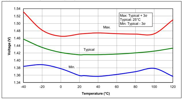
FIGURE 32-28: BROWN-OUT RESET VOLTAGE, BORV = 1
