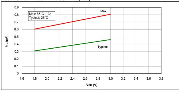
FIGURE 32-14: IPD, FIXED VOLTAGE REFERENCE (FVR)
