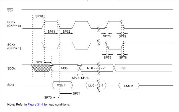
FIGURE 31-16: SPI MASTER MODE TIMING (CKE = 1, SMP = 1)
