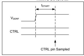
If the POR settings are satisfactory for the application, a microcontroller output pin can be freed by placing a weak pull-up or pull-down resistor on the CTRL pin. Only the DATA pin needs to be connected to an I/O pin.
