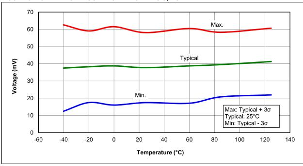
FIGURE 32-30: BROWN-OUT RESET VOLTAGE, BORV = 0
