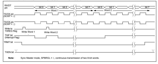
FIGURE 26-11: SYNCHRONOUS TRANSMISSION (THROUGH TXEN)
