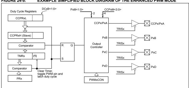
Note 1: The 8-bit timer TMRx register is concatenated with the 2-bit internal Q clock, or two bits of the prescaler to create the 10-bit time base.
