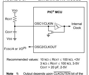
The RC oscillator frequency is a function of the supply voltage, the resistor (REXT) and capacitor (CEXT) values and the operating temperature. Other factors affecting the oscillator frequency are:
