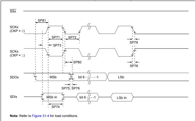
FIGURE 31-17: SPI SLAVE MODE TIMING (CKE = 0)
