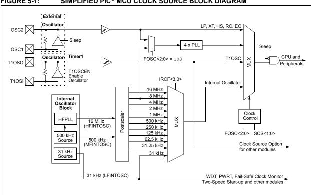
SIMPLIFIED PIC® MCU CLOCK SOURCE BLOCK DIAGRAM FIGURE 5-1:
