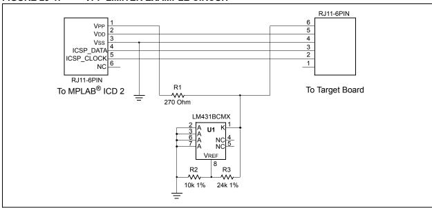
**Note:** The MPLAB ICD 2 produces a VPP voltage greater than the maximum VPP specification of the PIC16LF1824T39A.
