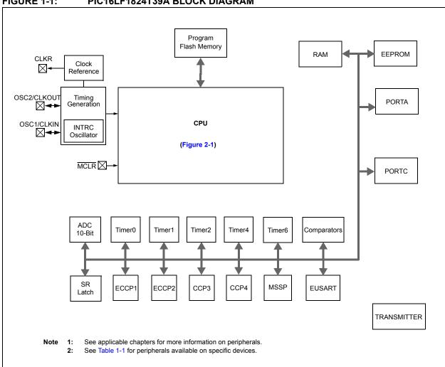
FIGURE 1-1: PIC16LF1824T39A BLOCK DIAGRAM
