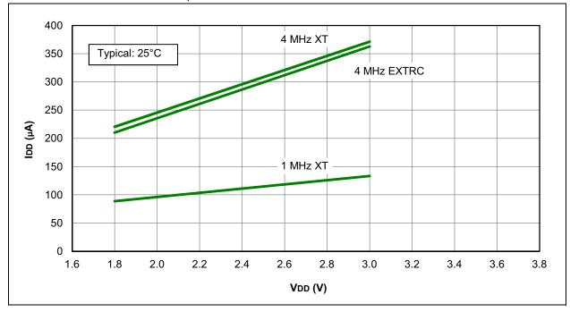
FIGURE 32-3: IDD MAXIMUM, XT AND EXTRC OSCILLATOR
