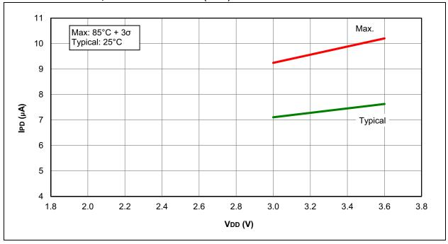
FIGURE 32-16: IPD, TIMER1 OSCILLATOR (Fosc = 32 kHz)
