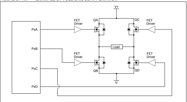
FIGURE 24-11: **EXAMPLE OF FULL-BRIDGE PWM OUTPUT**
