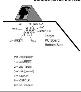
Another connector often found in use with the PICkit™ programmers is a standard 6-pin header with 0.1 inch spacing. Refer to Figure 29-3.
