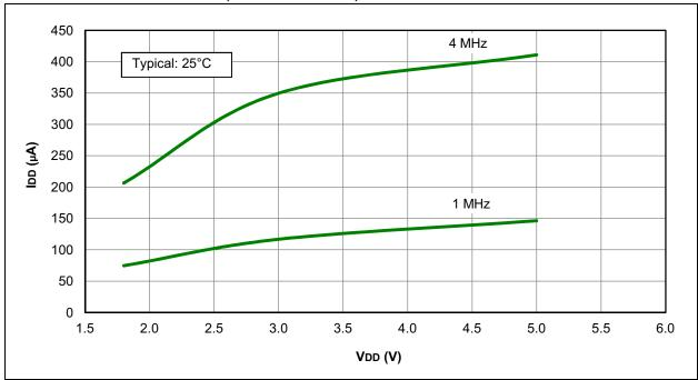
FIGURE 32-7: IDD, LFINTOSC MODE (Fosc = 31 kHz)
