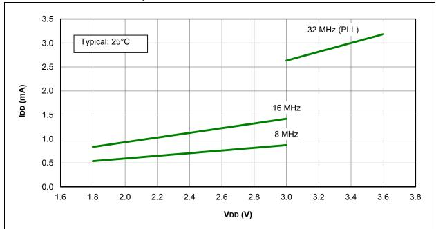
FIGURE 32-10: IDD MAXIMUM, HFINTOSC MODE
