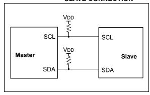
The Acknowledge bit  $(\overline{ACK})$  is an active-low signal, which holds the SDA line low to indicate to the transmitter that the slave device has received the transmitted data and is ready to receive more.
