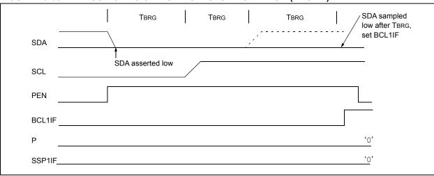
FIGURE 25-39: BUS COLLISION DURING A STOP CONDITION (CASE 2)
