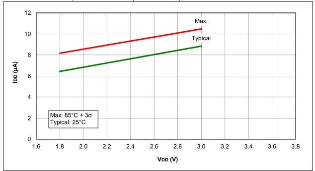
FIGURE 32-8: IDD, MFINTOSC MODE (Fosc = 500 kHz)
