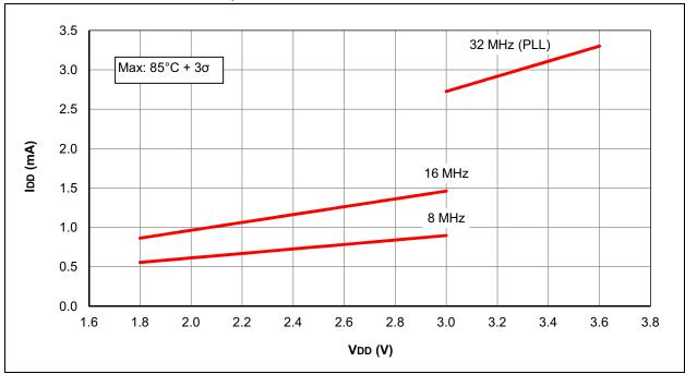
FIGURE 32-11: IDD, HS OSCILLATOR, 32 MHz (8 MHz + 4xPLL)
