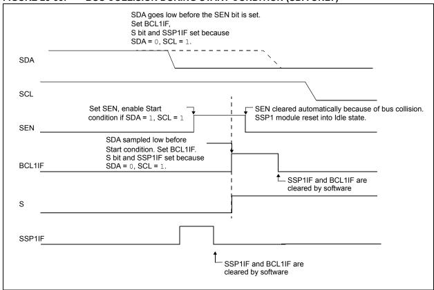
FIGURE 25-34: BUS COLLISION DURING START CONDITION (SCL = 0)
