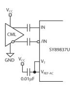
Figure 3d. CML Interface (AC-Coupled)
