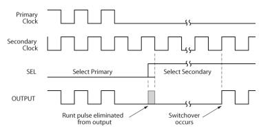
Figure 1. Simplified Example Illustrating Runt Pulse Eliminator (RPE)
