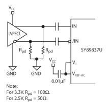
Figure 3b. LVPECL Interface (AC-Coupled)
