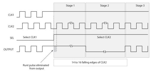
Figure 3. Timing Diagram 2<sup>(1)</sup>
