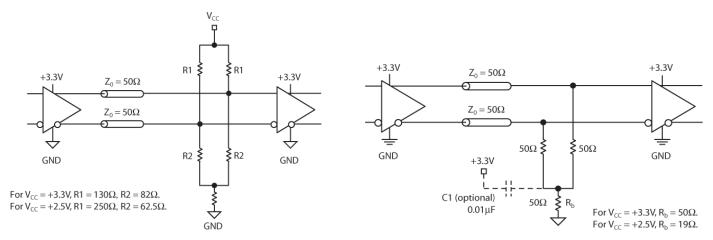
Figure 4a. Parallel Thevenin-Equivalent Termination
