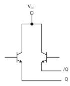
Figure 2b. Simplified LVPECL Output Stage
