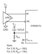
Figure 3a. LVPECL Interface (DC-Coupled)
