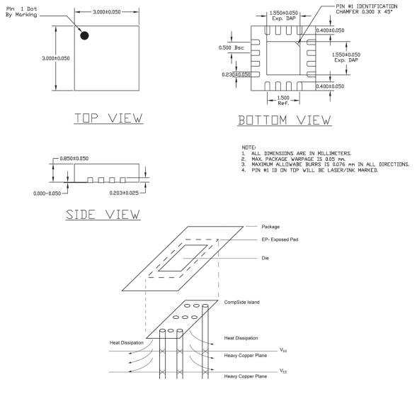
PCB Thermal Consideration for 16-Pin MLF<sup>®</sup> Package (Always solder, or equivalent, the exposed pad to the PCB)
