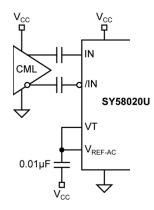
Figure 5. AC-Coupled CML Input Interface
