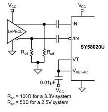
Figure 9. AC-Coupled LVPECL Input Interface
