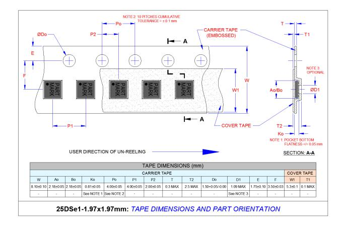
FIGURE 9-3: 25WLCSP, 1.97 X 1.97 REEL DIMENSIONS
