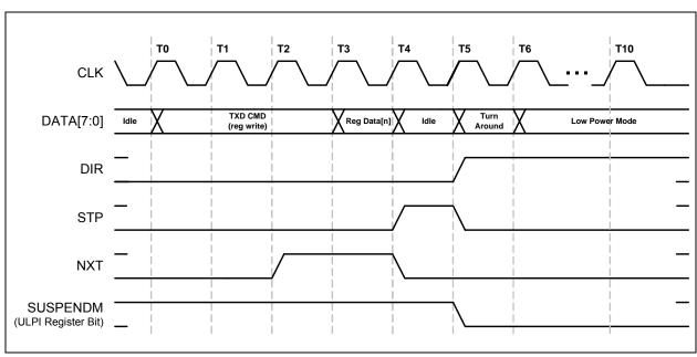
FIGURE 6-9: ENTERING LOW POWER MODE FROM SYNCHRONOUS MODE
