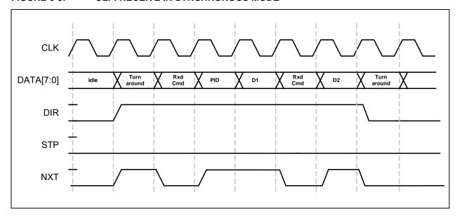
FIGURE 6-8: ULPI RECEIVE IN SYNCHRONOUS MODE
