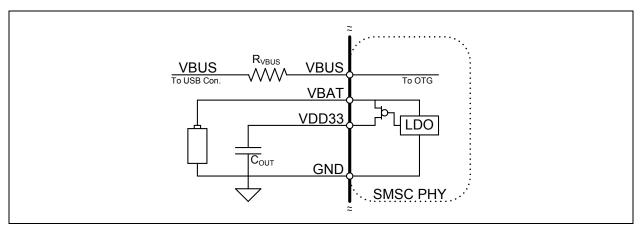
The USB332x can be powered from an external 3.3V supply as shown below in the Figure 5-6. When using the external supply, both the **VBAT** and **VDD33** pins are connected together. The bypass capacitor,  $C_{BYP}$ , should be included when using the external supply.
