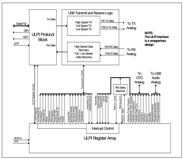
The advantage of a "wrapper less" architecture is that the USB332x has a lower USB latency than a design which must first register signals into the PHY's wrapper before the transfer to the PHY core. A low latency PHY allows a Link to use a wrapper around a UTMI Link and still make the required USB turn-around timing given in the USB 2.0 specification.
