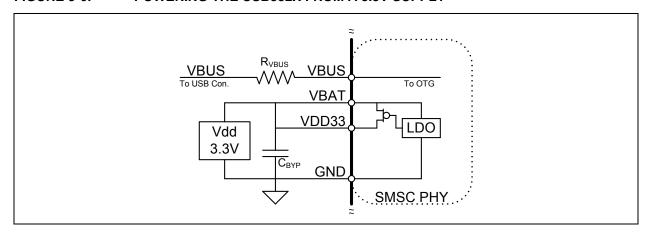
For peripheral only or host only operation, the **VBAT** supply shown below in Figure 5-7 may be connected to the **VBUS** pin of the USB connector for bus powered applications. In this configuration, external overvoltage protection is required to protect the **VBAT** supply from any transient voltage present at the **VBUS** pin of the USB connector.
