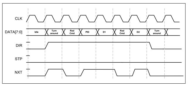
In Figure 6-8 the PHY asserts **DIR** to take control of the data bus from the Link. The assertion of **DIR** and **NXT** in the same cycle contains additional information that Rxactive has been asserted. When **NXT** is de-asserted and **DIR** is asserted, the RXCMD data is transferred to the Link. After the last byte of the USB receive packet is transferred to the PHY, the linestate will return to idle.
