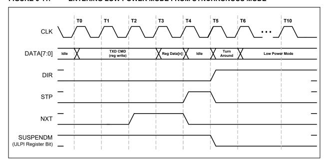
FIGURE 6-11: ENTERING LOW POWER MODE FROM SYNCHRONOUS MODE
