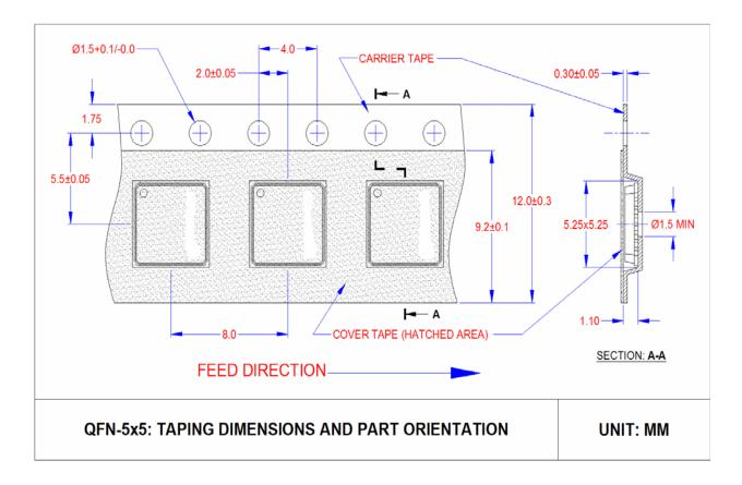
FIGURE 9-3: 32QFN, 5X5 REEL DIMENSIONS
