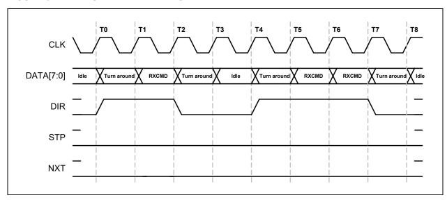
FIGURE 6-7: ULPI RXCMD TIMING
