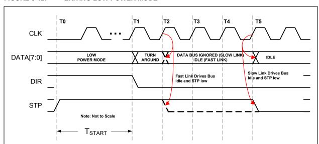
FIGURE 6-12: EXITING LOW POWER MODE
