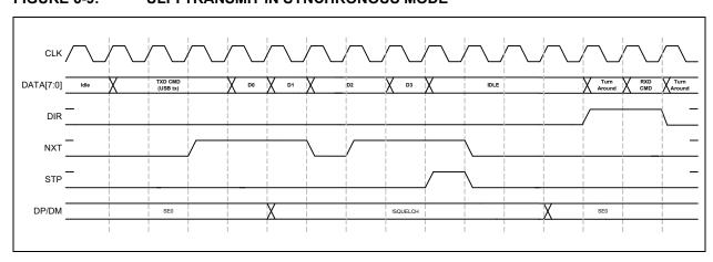
FIGURE 6-9: ULPI TRANSMIT IN SYNCHRONOUS MODE
