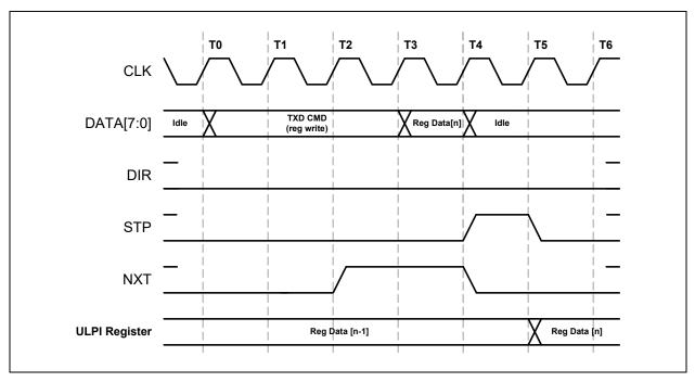
To write a register, the Link will wait until **DIR** is low, and at T0, drive the TX CMD on the data bus. At T2 the PHY will drive **NXT** high. On the next rising clock edge, T3, the Link will write the register data. At T4, the PHY will accept the register data and drive **NXT** low. The Link will drive an Idle on the bus and drive **STP** high to signal the end of the data packet. Finally, at T5, the PHY will latch the data into the register and the Link will pull **STP** low.
