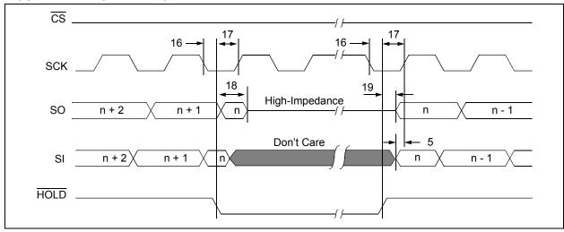
FIGURE 1-2: SERIAL INPUT TIMING
