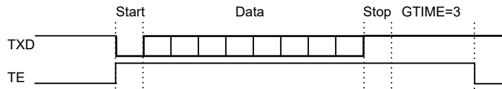
Figure 34-16. Example of TE Drive with Guard Time
