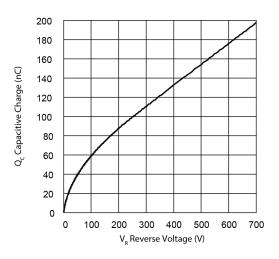
Figure 6 ● Total Capacitive Charge vs. V<sub>R</sub>
