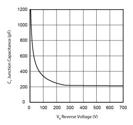
Figure 7 • Junction Capacitance vs  $V_R$
