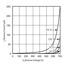
Figure 5 • Reverse Current vs. Reverse Voltage
