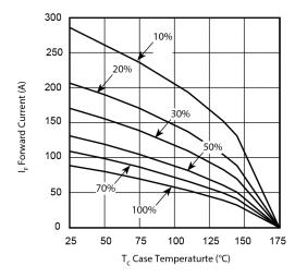
Figure 3 • Max Forward Current vs Case Temp
