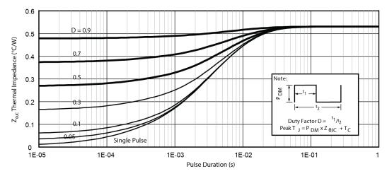
Figure 1 • Maximum Transient Thermal Impedance
