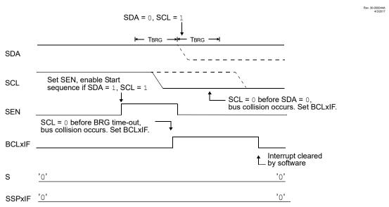
If the SDA pin is sampled low during this count, the BRG is reset and the SDA line is asserted early (see Figure 25-37). If, however, a '1' is sampled on the SDA pin, the SDA pin is asserted low at the end of the BRG count. The
