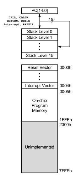
Figure 9-3. Program Memory and Stack (PIC16F15256/76)
