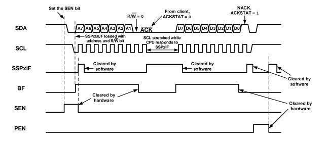
Figure 25-31. I<sup>2</sup>C Host Mode Waveform (Transmission, 10-Bit Address)
