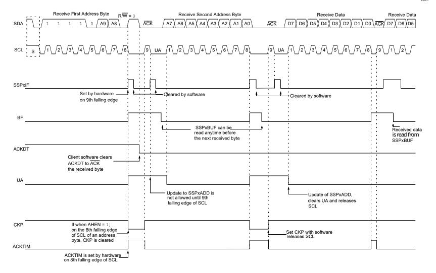
Figure 25-22. I<sup>2</sup>C Client, 10-Bit Address, Transmission (SEN = 0, AHEN = 0, DHEN = 0)
