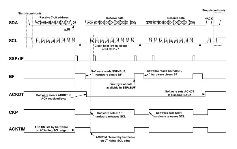
Figure 25-19. I<sup>2</sup>C Client, 7-Bit Address, Reception (SEN = 1, AHEN = 1, DHEN = 1)
