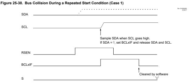
If SCL goes from high-to-low before the BRG times out and SDA has not already been asserted, a bus collision occurs. In this case, another host is attempting to transmit a data '1' during the Repeated Start condition (see Figure 25-39).
