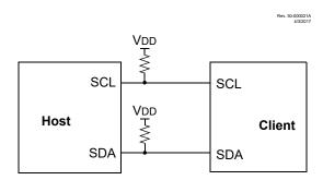
The I<sup>2</sup>C bus can operate with one or more host devices and one or more client devices.
