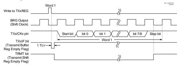
Figure 24-4. Asynchronous Transmission (Back-to-Back)
