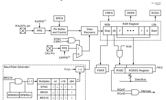
Figure 24-2. EUSART Receive Block Diagram
