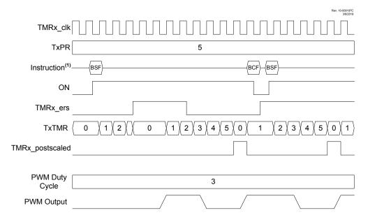
Note 1: BSF and BCF represent Bit-Set File and Bit-Clear File instructions executed by the CPU to set or clear the ON bit of TxCON. CPU execution is asynchronous to the timer clock input.
