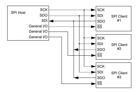
Transmissions involve two shift registers, eight bits in size: One in the host and one in the client. Data is always shifted out one bit at a time, with the Most Significant bit (MSb) shifted out first. At the same time, a new Least Significant bit (LSb) is shifted into the same register.
