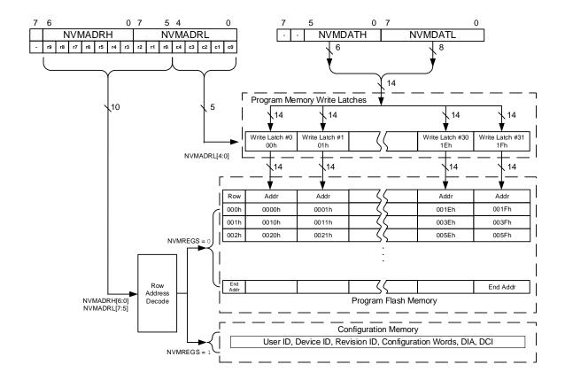
Figure 15-5. Program Flash Memory Write Sequence
