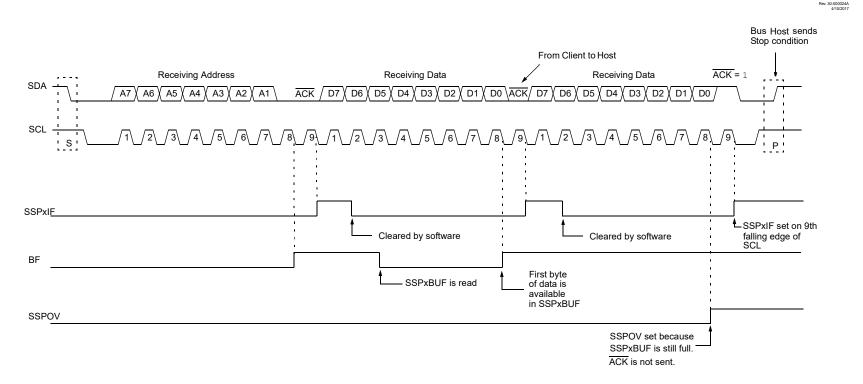
Figure 25-17. I<sup>2</sup>C Client, 7-Bit Address, Reception (SEN = 1, AHEN = 0, DHEN = 0)
