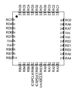
Note: It is recommended that the exposed bottom pad be connected to V<sub>SS</sub>; however, it must not be the only V<sub>SS</sub> connection to the device.
