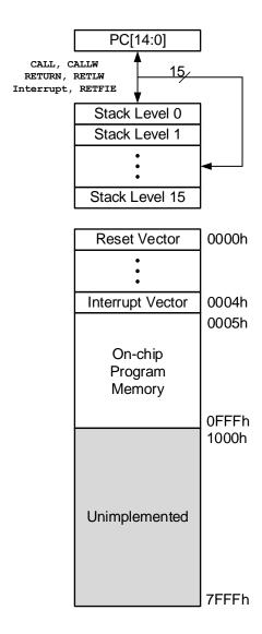
Figure 9-2. Program Memory and Stack (PIC16F15275)
