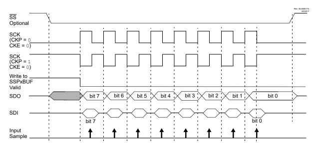
Figure 25-7. SPI Mode Waveform (Client Mode with CKE = 0)
