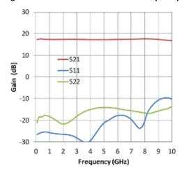
Figure 4 • Input Return Loss vs. Frequency
