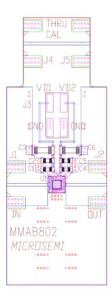
The circuit board used in the application should be generated with proper RF circuit design techniques. Signal lines at the RF ports should have 50  $\Omega$  impedance and the package ground leads and backside ground paddle should be connected directly to the ground plane similar to that shown previously.
