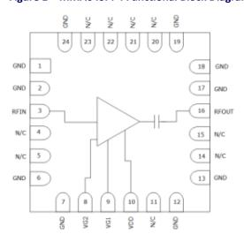
Figure 1 • MMA043PP4 Functional Block Diagram
