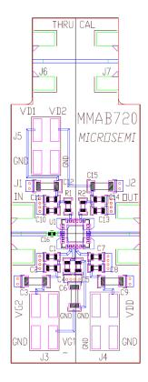
The circuit board used in the application should be generated with proper RF circuit design techniques. Signal lines at the RF port should have  $50~\Omega$  impedance, and the package ground leads and backside ground paddle should be connected directly to the ground plane similar to the previous image.
