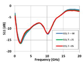
Figure 5 • Output Return Loss vs. Temperature
