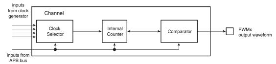
Each of the four channels is composed of three blocks:
