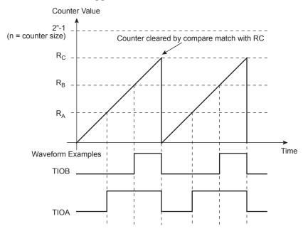
Figure 37-10: WAVSEL = 10 with Trigger
