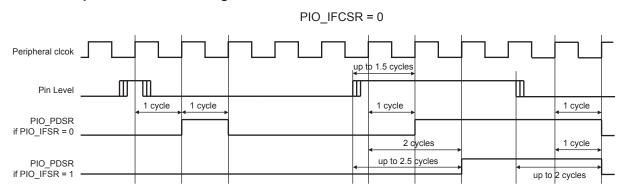
Figure 32-5: Input Debouncing Filter Timing
