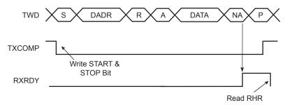
Figure 34-9: Master Read with Multiple Data Bytes
