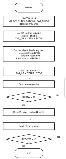
Figure 34-19: TWI Read Operation with Single Data Byte and Internal Address
