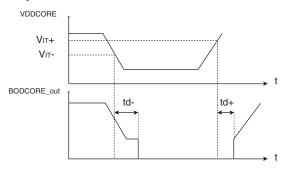
Figure 46-14: Core Brownout Transfer Characteristics
