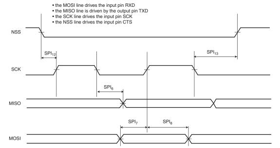
Figure 46-12: USART SPI Slave Mode: (Mode 0 or 3)
