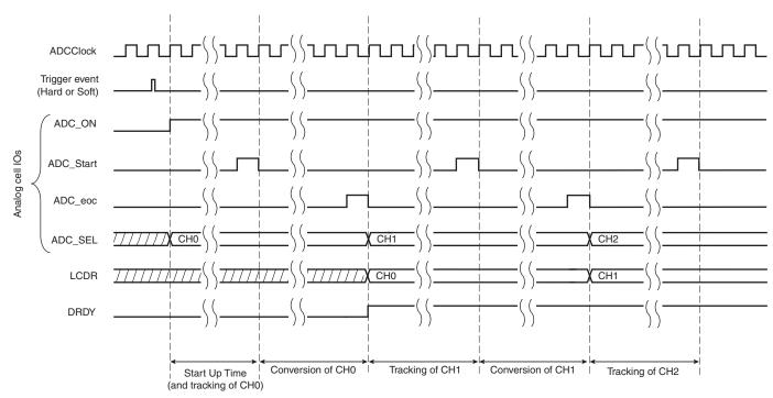
Figure 40-2: Sequence of ADC Conversions
