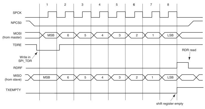
Figure 33-9 shows the behavior of Transmission Register Empty (TXEMPTY), End of RX buffer (ENDRX), End of TX buffer (ENDTX), RX Buffer Full (RXBUFF) and TX Buffer Empty (TXBUFE) status flags within the SPI\_SR during an 8-bit data transfer in Fixed mode with the PDC involved. The PDC is programmed to transfer and receive three units of data. The next pointer and counter are not used. The RDRF and TDRE are not shown because these flags are managed by the PDC when using the PDC.
