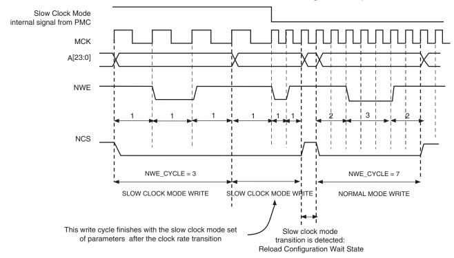
Figure 27-32: Recommended Procedure to Switch from Slow Clock Mode to Normal Mode or from Normal Mode to Slow Clock Mode
