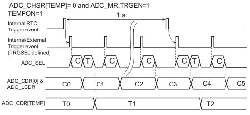
Notes: ADC\_SEL: Command to the ADC cell C: Classic ADC Conversion Sequence T: Temperature Sensor Channel
