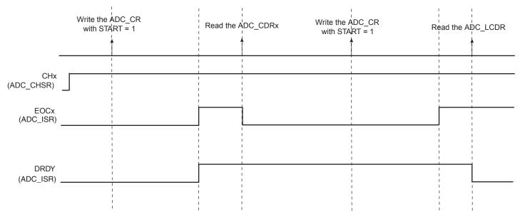
If ADC\_CDR is not read before further incoming data is converted, the corresponding Overrun Error (OVREx) flag is set in the Overrun Status register (ADC\_OVER).
