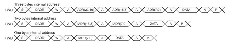
Figure 34-12: Master Read with One, Two or Three Bytes Internal Address and One Data Byte
