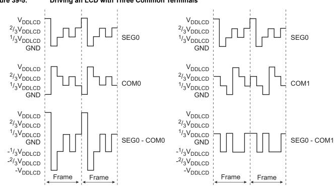
Figure 39-5: Driving an LCD with Three Common Terminals
