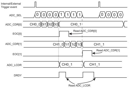
Notes: ADC\_SEL: Command to the ADC cell
