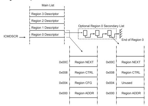
Figure 43-5 shows an example of the mandatory ICM settings to monitor three memory data blocks of the system memory (defined as two regions) with one region being not contiguous (two separate areas) and one contiguous memory area. For each said region, the SHA algorithm may be independently selected (different for each region). The wrap allows continuous monitoring.
