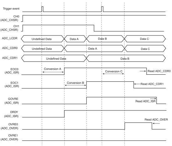
**Warning:** If the corresponding channel is disabled during a conversion or if it is disabled and then reenabled during a conversion, the associated data and the corresponding EOCx and GOVRE flags in ADC ISR and OVREx flags in ADC OVER are unpredictable.
