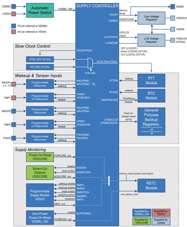
Note: TMPx signals and WKUPx signals are multiplexed on the same pins (e.g., TMP0/WKUP0, TMP1/WKUP10, etc.). This generates a wakeup event only, a tamper event only or a wakeup and a tamper event.
