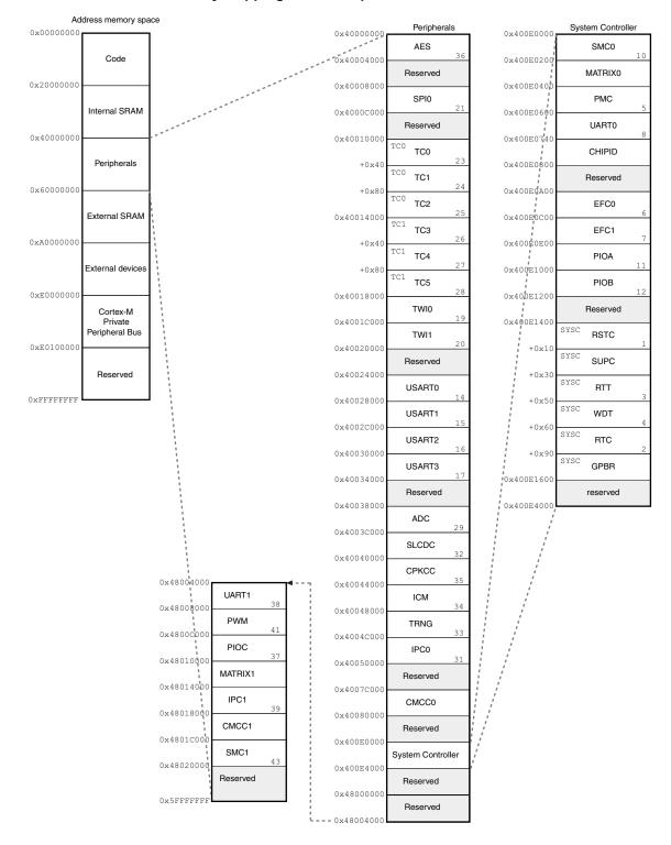
Figure 7-5: SAM4CM32 Memory Mapping of the Peripherals Area
