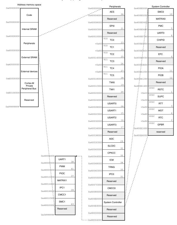
Figure 7-4: SAM4CM16/8/4 Memory Mapping of the Peripherals Area
