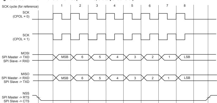
Figure 36-38: SPI Transfer Format (CPHA = 0, 8 bits per transfer)
