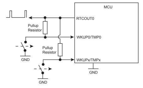
Figure 20-8: Low-power Debouncer (Push-to-Break Switch, Pulldown Resistors)
