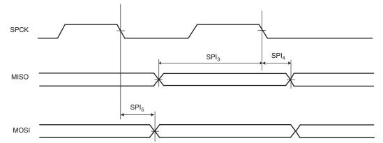
Figure 46-6: SPI Slave Mode with (CPOL=0 and NCPHA=1) or (CPOL=1 and NCPHA=0)
