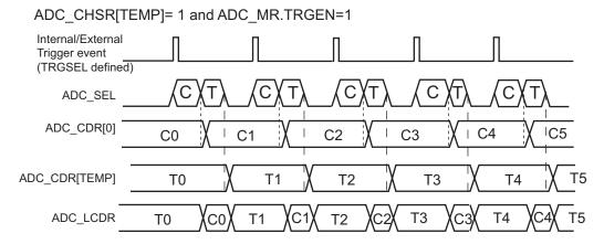
Notes: ADC\_SEL: Command to the ADC cell C: Classic ADC Conversion Sequence T: Temperature Sensor Channel
