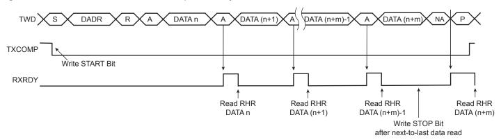
Figure 34-10: Master Read Wait State with Multiple Data Bytes
