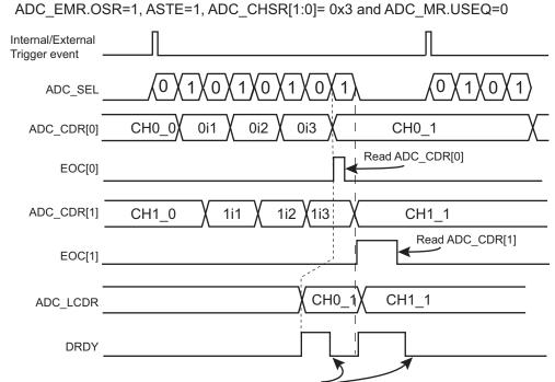
Notes: ADC\_SEL: Command to the ADC cell 0i1,0i2,0i3, 1i1, 1i2, 1i3 are intermediate results and CH0/1\_0/1 are final results of average function.
