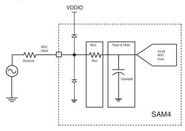
During its tracking phase, the 10-bit ADC charges its sampling capacitor through various serial resistors: source output resistor, multiplexer series resistor and the sampling switch series resistor. In case of high output source resistance (low power resistive divider, for example), the track time must be increased to ensure full settling of the sampling capacitor voltage. The following formulas give the minimum track time that guarantees a 10-bit accurate settling:
