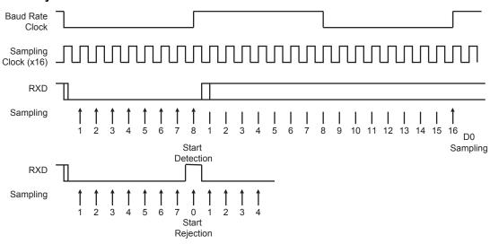
Figure 36-12: Asynchronous Character Reception
