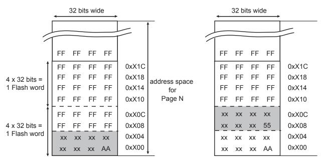
Step 1: Flash array after programming first byte (0xAA) 64-bit used at address 0xX00 (write latch buffer + WP)
