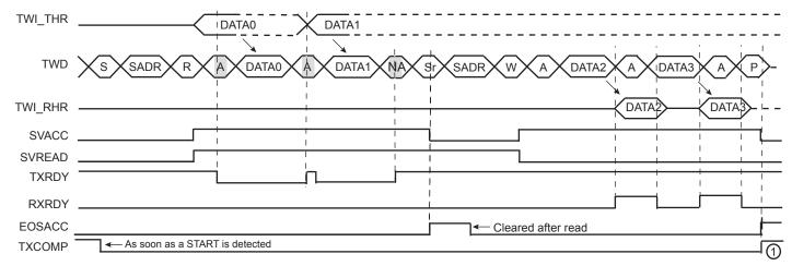
Note 1: TXCOMP is only set at the end of the transmission because after the repeated start, SADR is detected again.
