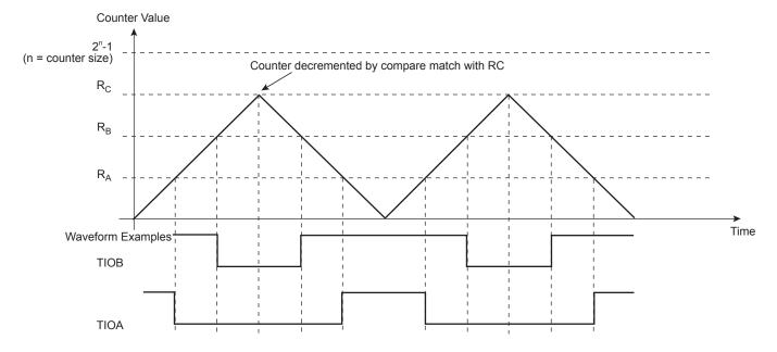
Figure 37-14: WAVSEL = 11 with Trigger
