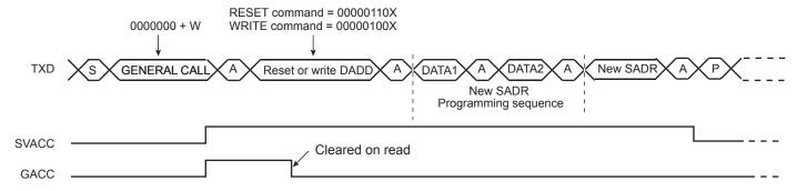
**Note:** This method allows the user to create a personal programming sequence by choosing the programming bytes and the number of them. The programming sequence has to be provided to the master.
