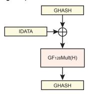
It is possible to process a message with only AAD setting the CLEN field to '0' in the AES\_CLENR, this can be used for  $J_0$  generation when len(IV)  $\neq$  96 for instance.
