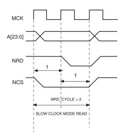
Table 27-6: Read and Write Timing Parameters in Slow Clock Mode
