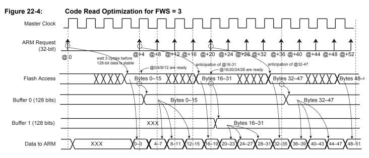
**Note:** When FWS is between 1 and 3, in case of sequential reads, the first access takes (FWS + 1) cycles. The following accesses take only one cycle.
