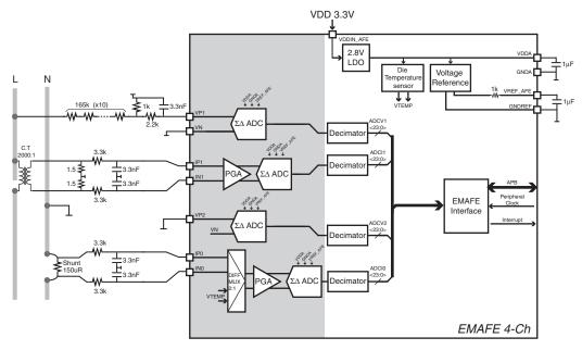
Example Application Diagram for EMAFE in a Typical 100A (Imax), single-phase with anti-tamper Smart Meter
