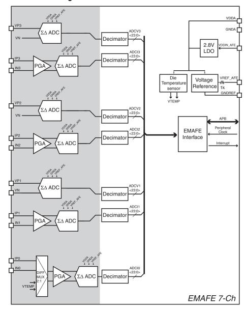
Figure 41-2: Functional Block Diagram for Two-Phase EMAFE
