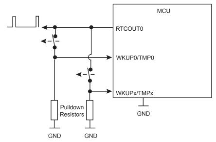
The duration of the debouncing period is configurable. The period is identical for all debouncers (i.e., the duration cannot be adjusted separately for each debouncer). The number of successive identical samples to wake up the system can be configured from 2 up to 8 in the LPDBC field of SUPC\_WUMR. The period of time between two samples can be configured in the TPERIOD field in the RTC\_MR. Power parameters can be adjusted by modifying the period of time in the THIGH field in RTC\_MR.
