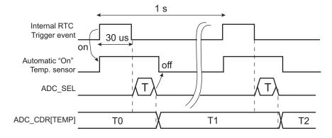
Notes: ADC\_SEL: Command to the ADC cell C: Classic ADC Conversion Sequence T: Temperature Sensor Channel It is possible to raise a flag only if there is a predefined change in the temperature. The user can define a range of temperature or a threshold in the Temperature Compare Window register (ADC\_TEMPCWR), and the mode of comparison that can be programmed into the TEMPCMPMOD field into ADC\_TEMPMR. These values define how the TEMPCHG flag is raised in ADC\_ISR.
