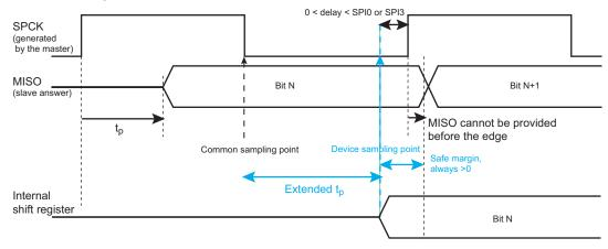
Figure 46-4: SPI Master Mode with (CPOL= NCPHA = 0) or (CPOL= NCPHA= 1)
