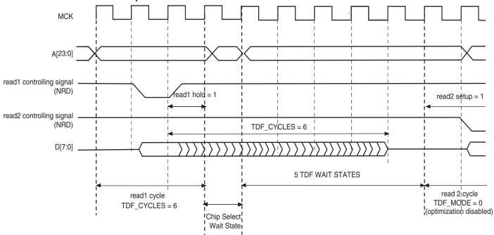
Figure 27-23: TDF Mode = 0: TDF wait states between a read and a write access on different chip selects
