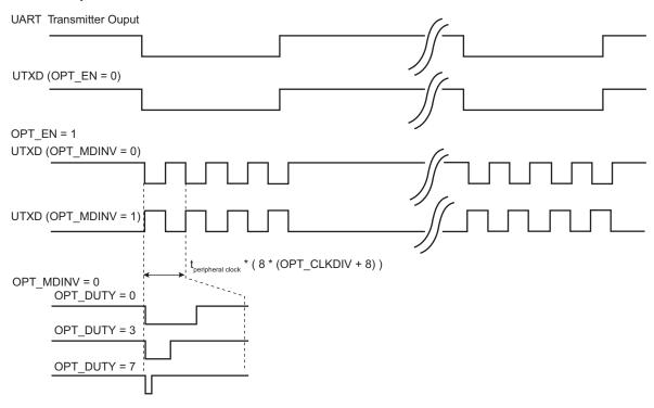
The default configuration values of the optical link circuitries allow the 38 kHz modulation, a 50% duty cycle and an idle polarity allowing a direct drive of an IR LED through a resistor (see Figure 35-13).
