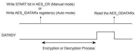
If the user does not want to read the AES\_ODATARx between each encryption/decryption, the DATRDY flag will not be cleared. If the DATRDY flag is not cleared, the user cannot know the end of the following encryptions/decryptions.
