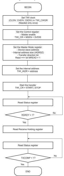
Figure 34-20: TWI Read Operation with Multiple Data Bytes with or without Internal Address
