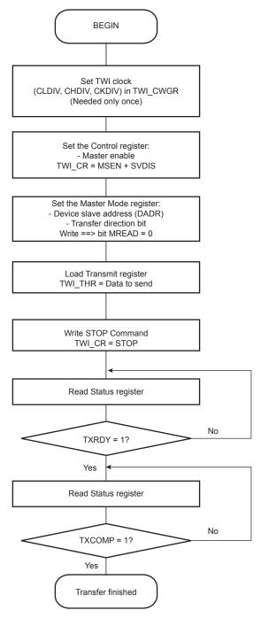
Figure 34-16: TWI Write Operation with Single Data Byte and Internal Address
