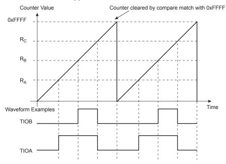
Figure 37-8: WAVSEL = 00 with Trigger
