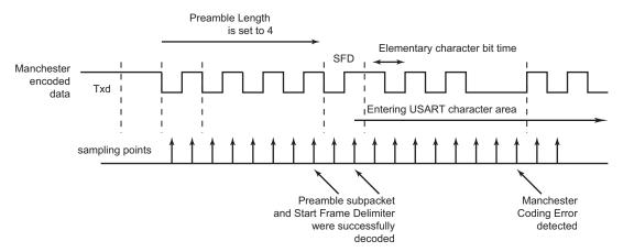
When the start frame delimiter is a sync pattern (ONEBIT field to 0), both command and data delimiter are supported. If a valid sync is detected, the received character is written as RXCHR field in the US\_RHR and the RXSYNH is updated. RXCHR is set to 1 when the received character is a command, and it is set to 0 if the received character is a data. This mechanism alleviates and simplifies the direct memory access as the character contains its own sync field in the same register.
