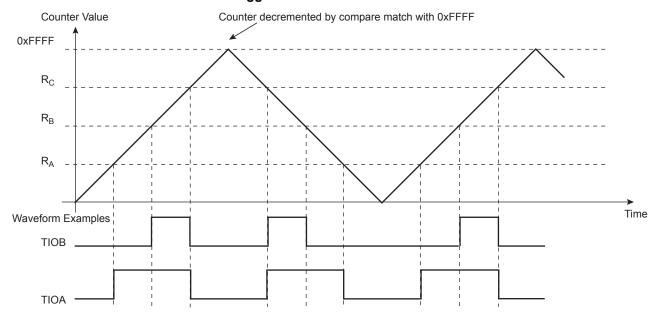
Figure 37-12: WAVSEL = 01 with Trigger
