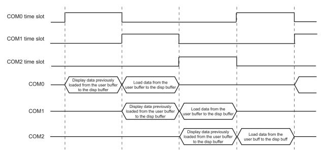
When a bit in the display memory (SLCDC\_LMEMRx and SLCDC\_MMEMRx registers) is written to one, the corresponding segment is energized (on), and non-energized when a bit in the display memory is written to zero.
