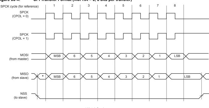
Figure 33-4: SPI Transfer Format (NCPHA = 0, 8 bits per transfer)
