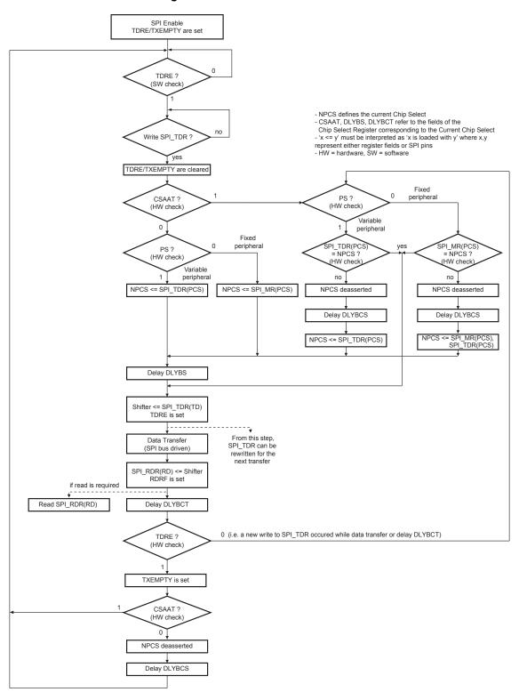
Figure 33-8 shows the behavior of Transmit Data Register Empty (TDRE), Receive Data Register (RDRF) and Transmission Register Empty (TXEMPTY) status flags within the SPI\_SR during an 8-bit data transfer in Fixed mode without the PDC involved.
