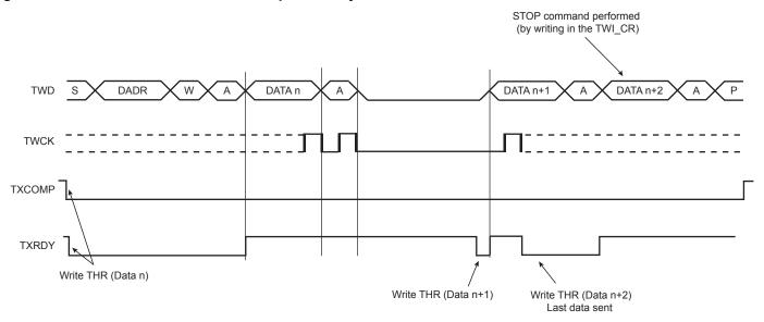
Figure 34-7: Master Write with One Byte Internal Address and Multiple Data Bytes
