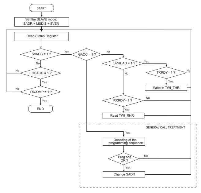
Figure 34-32: Read Write Flowchart in Slave Mode
