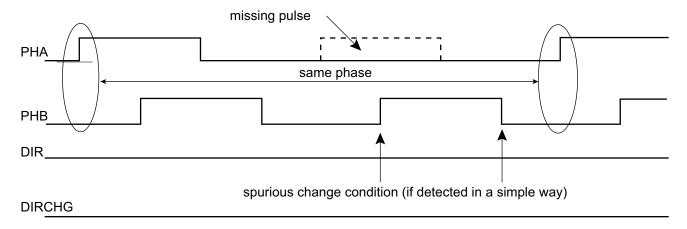
The direction change detection is disabled when QDTRANS is set in the TC BMR. In this case, the DIR flag report must not be used.
