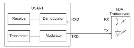
The receiver and the transmitter must be enabled or disabled depending on the direction of the transmission to be managed.
