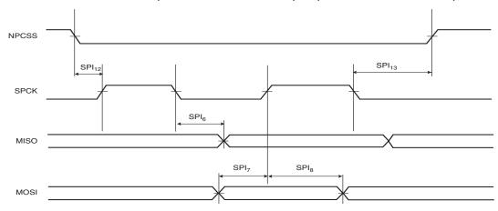
Figure 46-7: SPI Slave Mode with (CPOL = NCPHA = 0) or (CPOL= NCPHA= 1)
