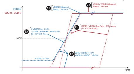
Table 46-4: Recommended Operating Conditions on Power Supply Inputs at Powerup
