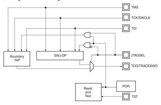
Figure 13-2 illustrates the dual core debug implementation using only one SW-JTAG/SW-DP Debug Access Port. Star topology has been used to connect the AHB-AP 0 (Core 0) and AHB-AP 1 (Core) rather than legacy daisy-chaining method. Star topology provides higher performance than daisy-chain topology. This core debug architecture is fully supported by debug tools vendors.
