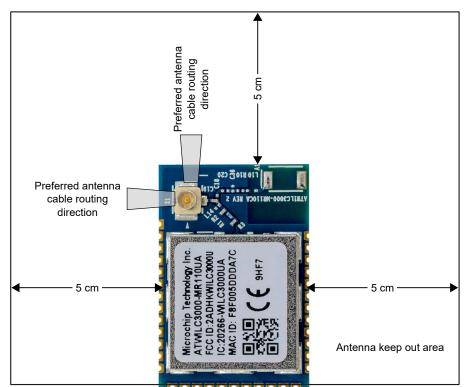
**Note:** These are generic guidelines and it is recommended that customers check and fine-tune the antenna positioning in the final host product based on RF performance.
