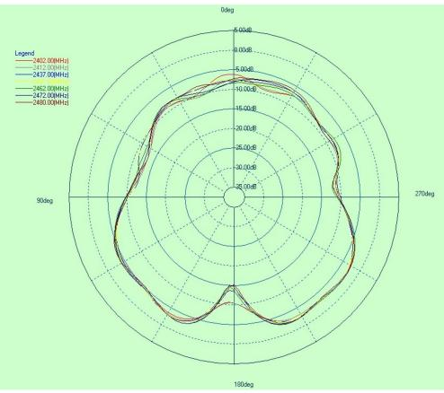
Figure 13-4. Antenna Radiation Pattern When Phi = 90 Degrees
