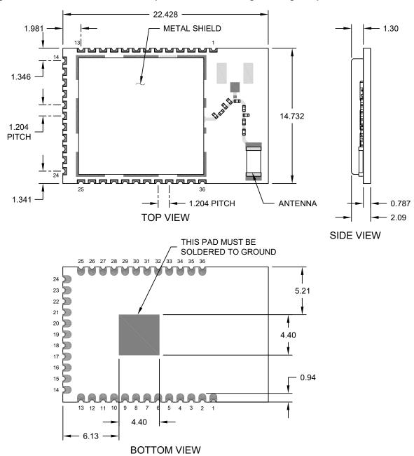
Figure 12-2. ATWILC3000-MR110CA Module Package Drawings - 3D View and Recommended Land Pattern
