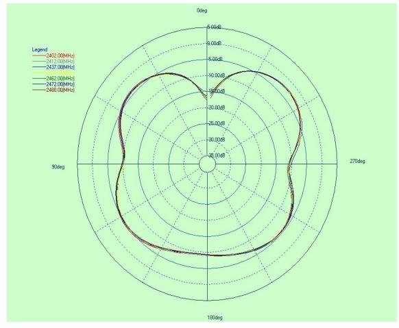
Figure 13-5. Antenna Radiation Pattern When Theta = 90 Degrees
