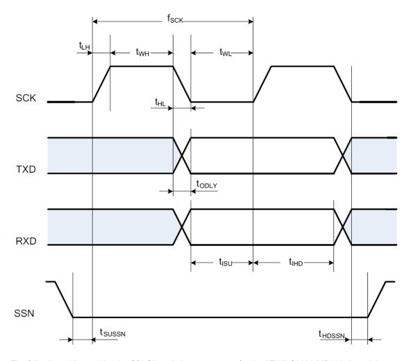
The following table provides the SPI Client timing parameters for the ATWILC3000-MR110xA module.
