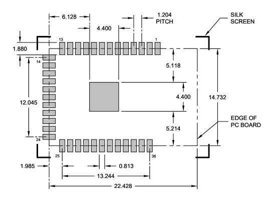
Figure 12-3. ATWILC3000-MR110UA Footprint and Module Package Drawings - Top, Bottom and Side View
