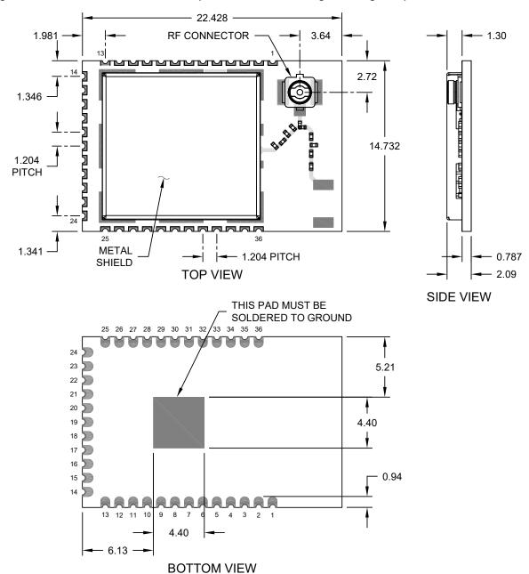
Figure 12-4. ATWILC3000-MR110UA Module Package Drawings - 3D View and Recommended Land Pattern
