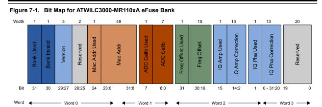
**Note:** The bit map was updated with bit fields IQ Amp correction and IQ Pha Correction fields from the firmware version 15.3 for WILC Linux and 4.5 for WILC RTOS onwards. Earlier, these bit fields were reserved for future use. For customers using firmware older than 15.3 for WILC Linux and 4.5 for WILC RTOS, IQ Amp correction and IQ Pha Correction bit fields will not be used by the firmware.
