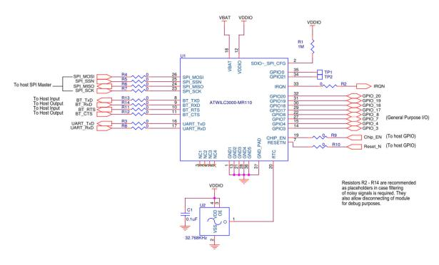
Note: Adding test points for module pins 8, 9, 10, 11, 16 and 17 in the design is recommended.
