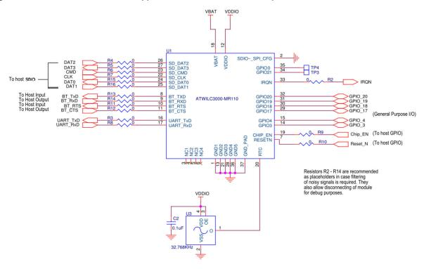
Note: Adding test points for module pins 8, 9, 10, 11, 16 and 17 in the design is recommended.
