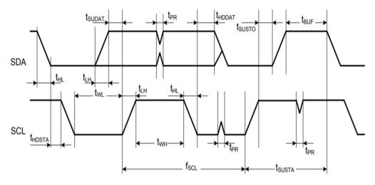
The following table provides the I<sup>2</sup>C Client timing parameters for the ATWILC3000-MR110xA module.
