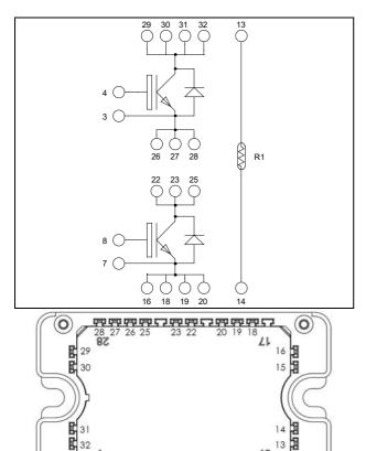
Pins 29/30/31/32 must be shorted together Pins 26/27/28/22/23/25 must be shorted together to achieve a phase leg Pins 16/18/19/20 must be shorted together
