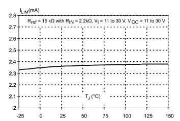
Figure 10. Typical limiting current  $I_{LIM}$  versus junction temperature  $T_j$
