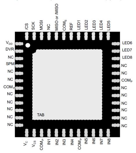
Figure 3. Pinout description of the QFN7x7-48L version (top view)
