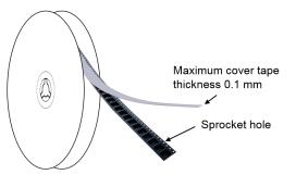
Figure 13. Reel dimension values (mm)
