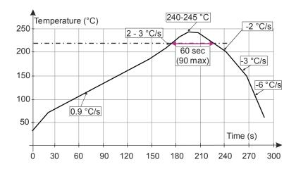
Note: Minimize air convection currents in the reflow oven to avoid component movement. Maximum soldering profile corresponds to the latest IPC/JEDEC J-STD-020.
