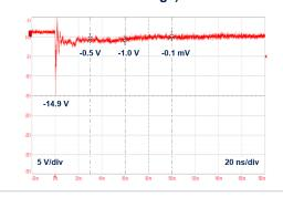
Figure 7. ESD response to IEC 61000-4-2 (+8 kV contact discharge)
