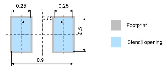
Stencil opening thickness: 100 µm
