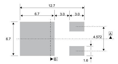
Figure 21. DPAK recommended footprint (dimensions are in mm)
