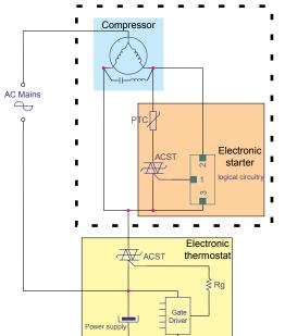
Compressor with integrated e-starter
