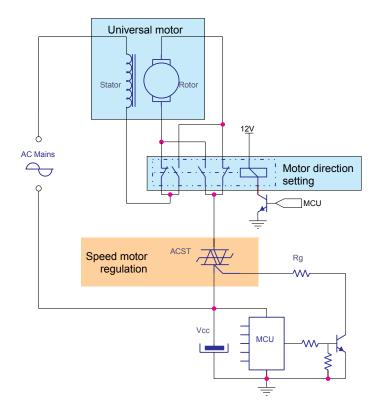
Figure 16. Universal drum motor control – typical diagram
