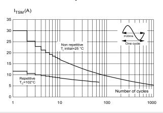
Figure 8. Non repetitive surge peak on-state current for a sinusoidal pulse width
