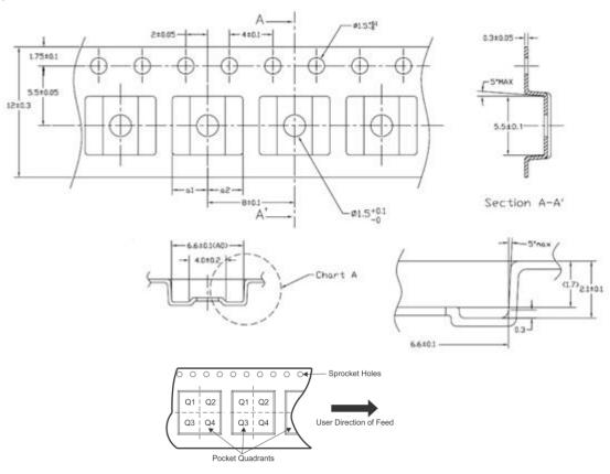
Note: The Pin 1of the chip is in the quadrant Q1
