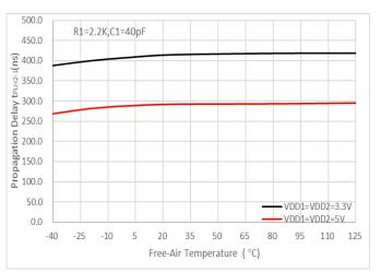
Figure 14. tplh2-1 Propagation Delay vs Free-Air Temperature
