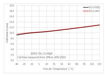
Figure 7. Side 1: Output Fall Time vs Free-Air Temperature
