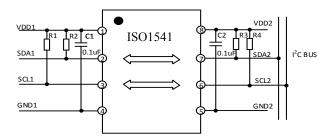
Figure 2. ISO1541 Typical Application Circuit
