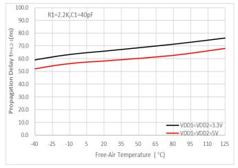
Figure 15. tphl2-1 Propagation Delay vs Free-Air Temperature
