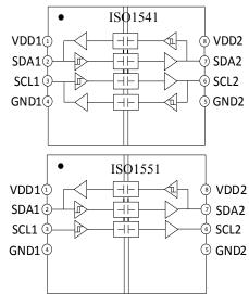
Figure 1. ISO1541/1551 functional Block Diagram
