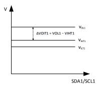
Figure 21. ISO1541/1551 side 1 voltage Diagram
