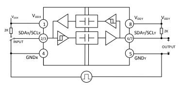
Figure 19. Common-Mode Transient Immunity Test Circuit
