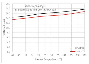
Figure 9. Side 2: Output Fall Time vs Free-Air Temperature
