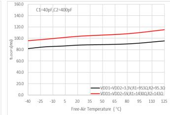
Figure 16. tloop1 vs Free-Air Temperature
