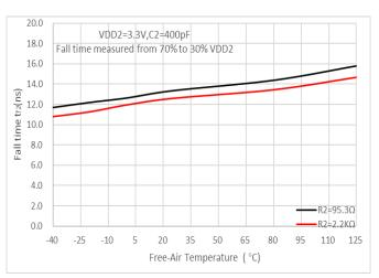
Figure 8. Side 2: Output Fall Time vs Free-Air Temperature
