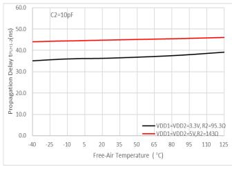
Figure 10. tplh1-2 Propagation Delay vs Free-Air Temperature
