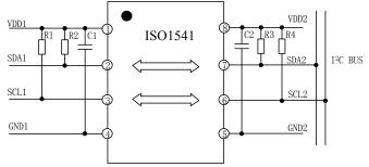
Figure 22. Typical Isolated I<sup>2</sup>C Interface Using the ISO1541
