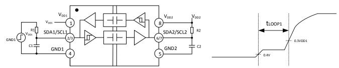
Figure 18. tLoop1 Setup and Timing Diagram
