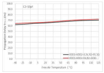
Figure 11. tphl1-2 Propagation Delay vs Free-Air Temperature
