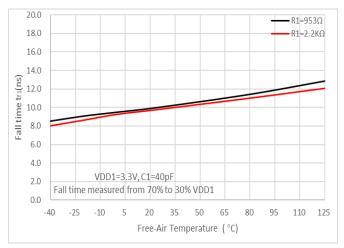
Figure 6. Side 1: Output Fall Time vs Free-Air Temperature
