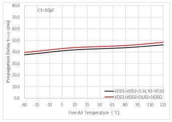
Figure 12. tplh1-2 Propagation Delay vs Free-Air Temperature
