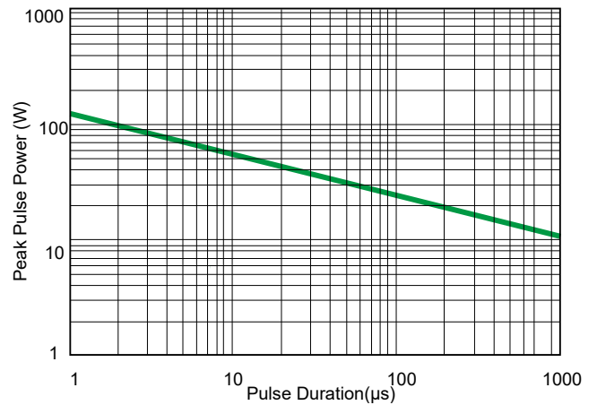
Fig 6. Non Repetitive Peak Pulse Power vs. Pulse time
