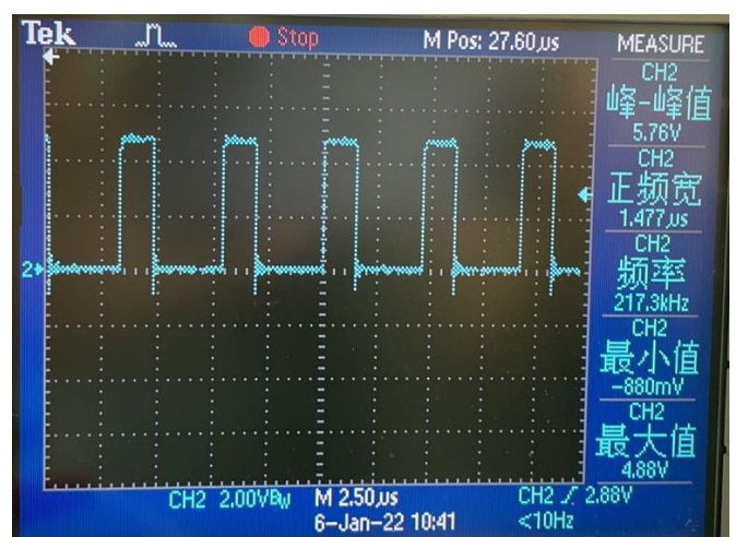
MOS switch waveform
