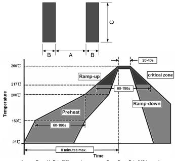
Average Ramp-Up Rate:3°C/second max. Ramp-Down Rate:6 °C /second max
