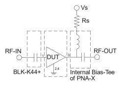
Fig 1. Characterization Circuit
