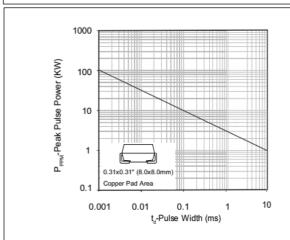
Figure 3. Peak pulse power rating curve
