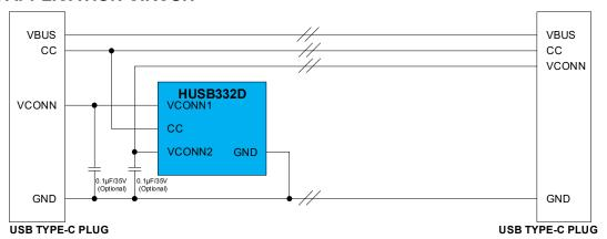
Figure 1. HUSB332D\_UXXDH Typical Application Circuit
