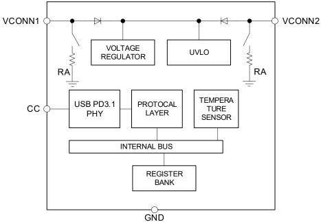
Figure 4. HUSB332D Functional Block Diagram
