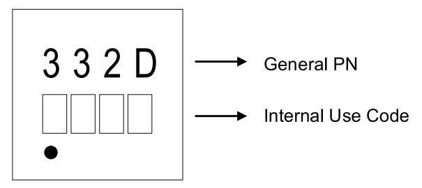
Figure 11. DFN1.6×1.6-4L& DFN2×2-6L Package Top Marking
