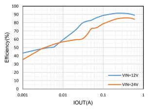
Figure 1. Efficiency vs Load Current, Vout=5V
