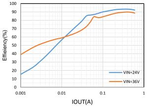
Figure 2. Efficiency vs Load Current, Vout=12V
