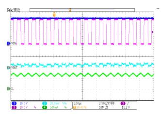
Figure 20.Load Transient (0.06A-0.54A, 250mA/us)
