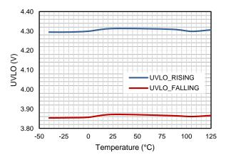
Figure 11. VIN UVLO VS Temperature
