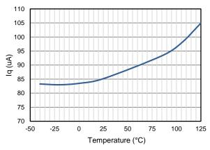
Figure 8. Quiescent Current vs Temperature VIN=12V
