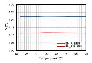
Figure 10. EN Threshold vs Temperature
