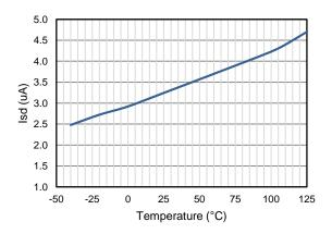
Figure 9. Shutdown Current vs Temperature, Vin=24V
