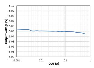
Figure 4. Load Regulation (Vout=5V), Vin=24V
