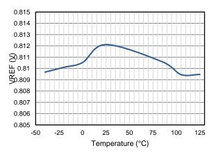
Figure 5. Reference VS Temperature
