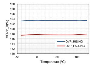
Figure 12. OVP VS Temperature
