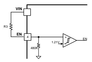
Figure 14. Adjustable VIN UVLO
