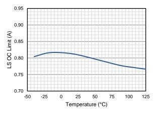
Figure 7. LS Current Limit VS Temperature
