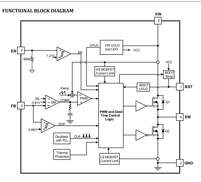
Figure 13. Functional Block Diagram
