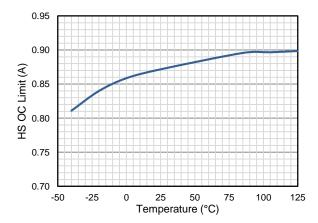
Figure 6. HS Current Limit VS Temperature
