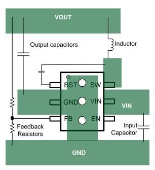
Figure 24. PCB Layout Example
