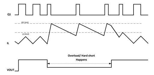
Figure 15 Over Current Protection
