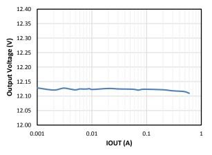
Figure 3. Load Regulation (Vout=12V), Vin=24V
