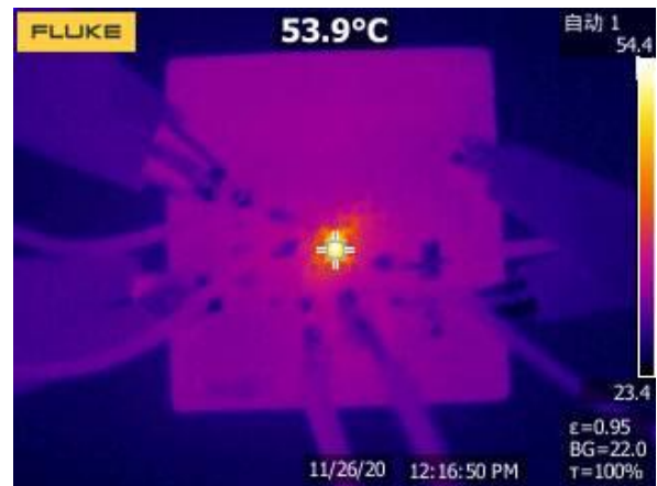
Figure 23. Thermal, 24VIN, 12Vout, 0.6A
