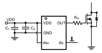
Figure 24. NCP81071 Inverting MOSFET Gate Drive Typical Application
