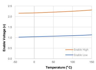
Figure 4. Enable Threshold vs Temperature
