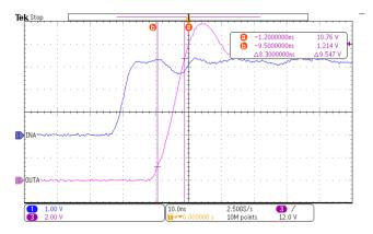
Figure 17. Driver Switching ON
