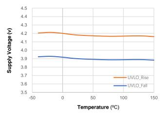
Figure 1. UVLO vs Temperature
