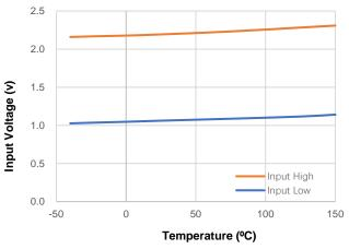
Figure 3. Input Threshold vs Temperature
