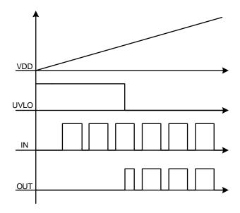
Figure 11. NCP81071 Output Vs VDD
