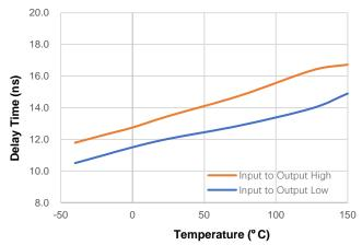
Figure 7. Input to Output Propagation Delay vs Temperature
