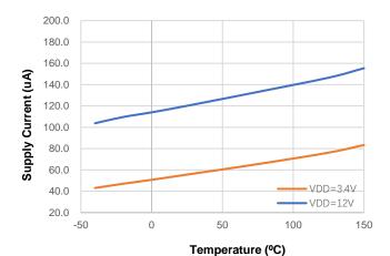
Figure 2. Start-up current vs Temperature
