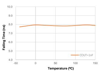
Figure 6. Output Falling Time vs Temperature
