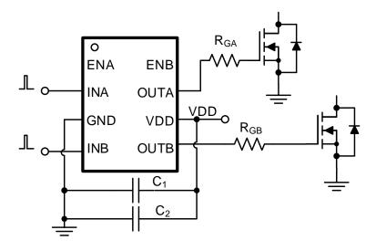
Figure 16. Dual Channel Driver Typical Application
