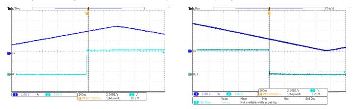
Figure 14. Driver Switching ON
