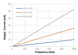
Figure 10. Operation Supply Current vs Frequency, Cout=1nF
