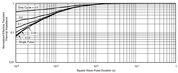
Normalized Thermal Transient Impedance, Junction-to-Case
