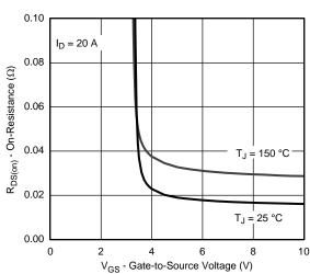
On-Resistance vs. Gate-to-Source Voltage
