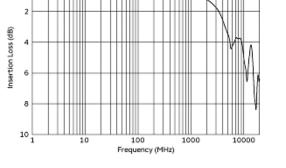
**Common Mode Insertion Loss Characteristic** (Typical Value)
