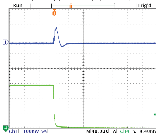
Step Load Transient Response (Vin=12V, Vout=5V, Cload=12x10μF X5R 0805 ceramic, total 120μF, Iout=3A to 0A) Top trace=Vout, Bottom trace=Iout
