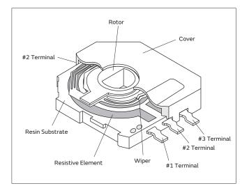
Heat both the terminal and the land at the same time so that the wire solder melts quickly. This will reduce deformation of the resin substrate of the product due to heat transmitted from the terminals.
