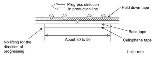
b) When hold down tape is spliced
