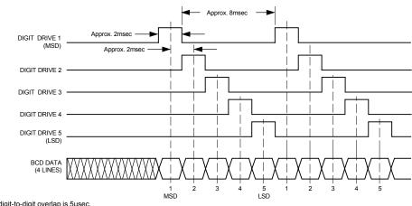
1. Maximum allowable digit-to-digit overlap is 5µsec. 2. Maximum allowable digit-to-BCD data skew is also 5µsec.
