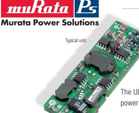
The ULE Series "Eighth-Brick" DC-DC Converters are high-current isolated power converters designed for use in high-density system boards.
