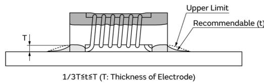
An increased solder volume increases mechanical stress on the product. Exceeding solder volume may cause the failure of mechanical or electrical performance.
