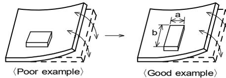
(2) Components location on PCB separation
