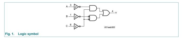
Low-power configurable multiple function gate
