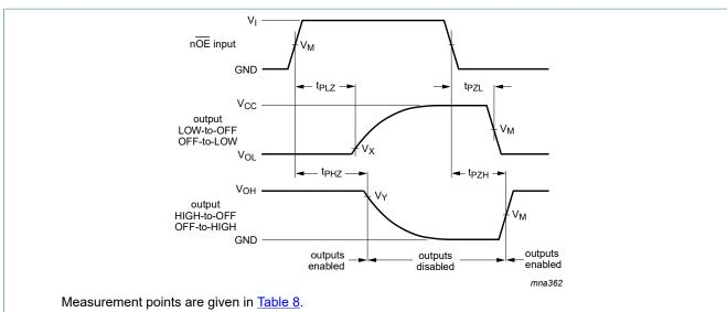
$V_{\text{OL}}$  and  $V_{\text{OH}}$  are typical voltage output levels that occur with the output load.
