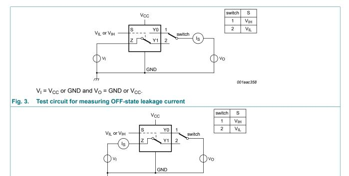
$V_I = V_{CC}$  or GND and  $V_O =$  open circuit.
