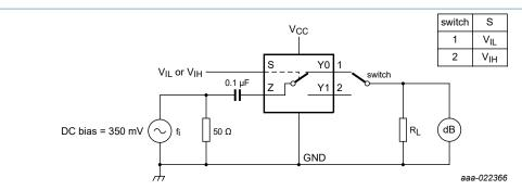
Adjust f<sub>i</sub> voltage to obtain 0 dBm level at output. Increase f<sub>i</sub> frequency until dB meter reads -3 dB.
