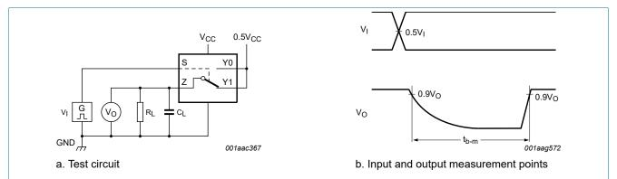
Fig. 14. Test circuit for measuring break-before-make timing
