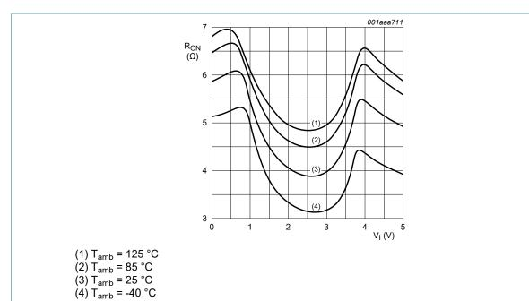
Fig. 11. ON resistance as a function of input voltage;  $V_{CC} = 5.0 \text{ V}$
