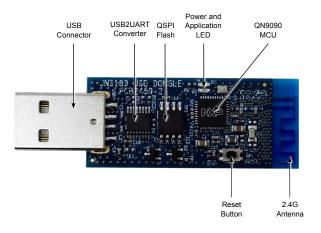
Figure 1: OM15080-QN9090 Board Components
