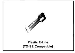
The E-line package is formed by transfer moulding a silicone plastic specially selected to provide a rugged one-piece encapsulation resistant to severe environments and allow the high junction temperature operation normally associated with metal can devices.
