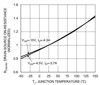
Figure 6. On-Resistance Variation with Temperature
