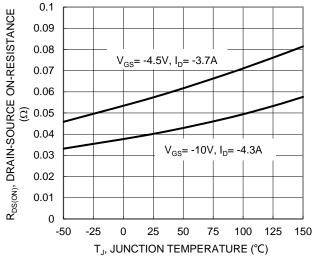
Figure 7. On-Resistance Variation with Temperature
