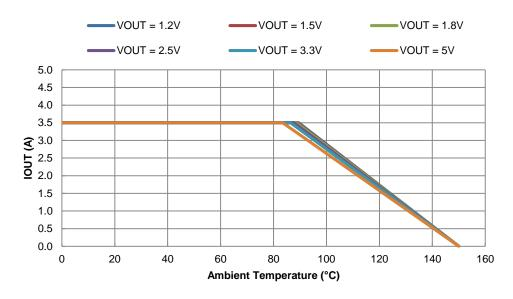
Figure 24. Output Current Derating Curve vs. Ambient Temperature, VIN = 12V, f<sub>SW</sub> = 500kHz
