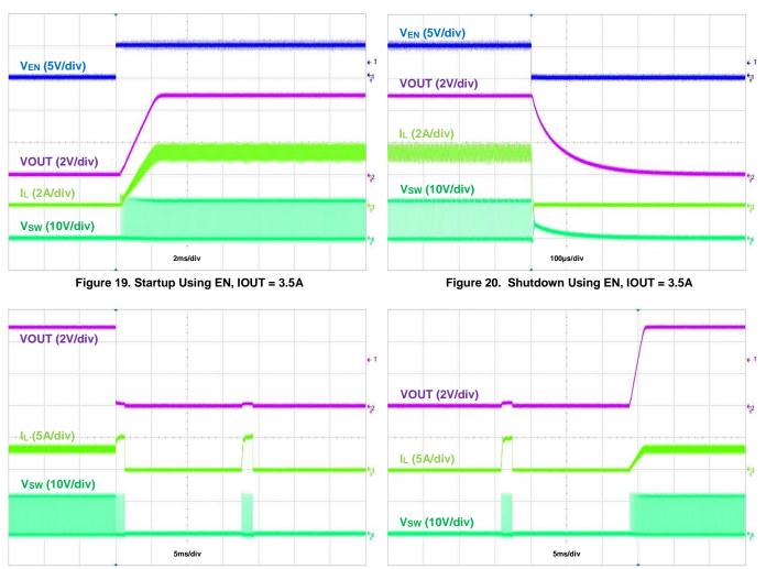
Figure 21. Output Short Protection, IOUT = 3.5A
