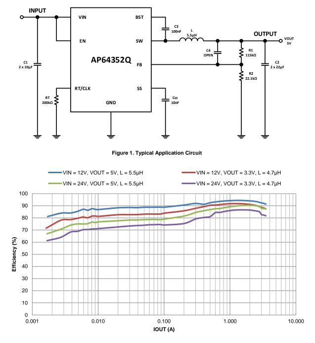
Figure 2. Efficiency vs. Output Current
