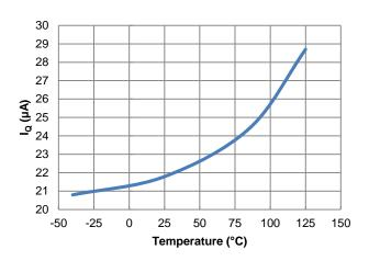
Figure 10. Io vs. Temperature
