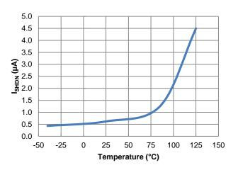
Figure 11. ISHDN vs. Temperature
