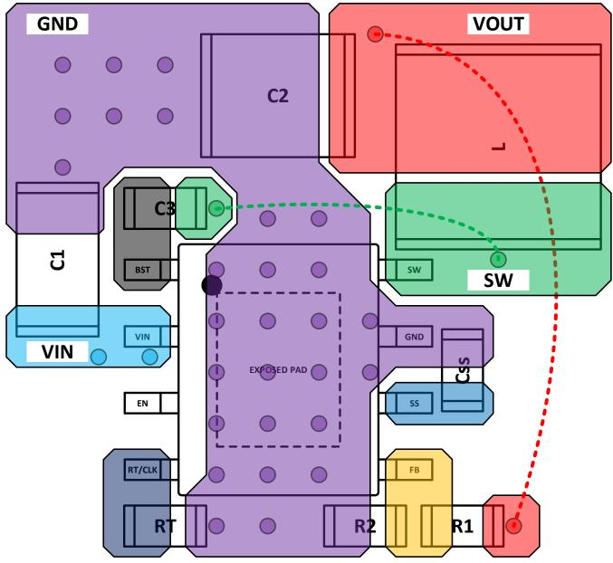
Figure 26. Recommended PCB Layout
