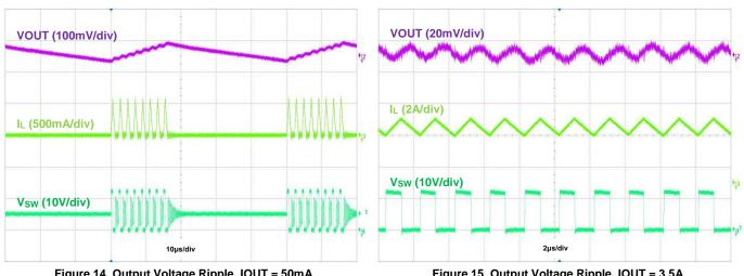
Figure 14. Output Voltage Ripple, IOUT = 50mA
