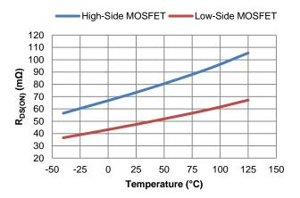
Figure 9. Power MOSFET RDS(ON) vs. Temperature
