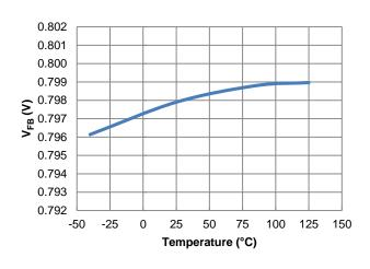
Figure 8. Feedback Voltage vs. Temperature
