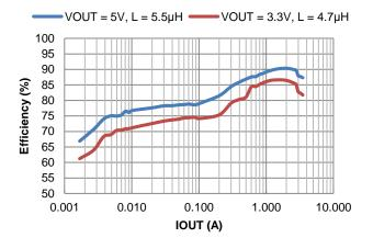
Figure 5. Efficiency vs. Output Current, VIN = 24V
