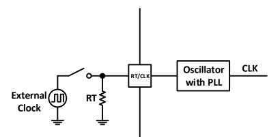
Figure 25. Switching Between Resistor Timing and External Clock Synchronization Modes
