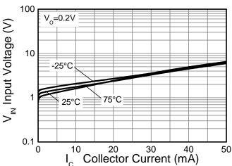
**Input Voltage v Collector Current**
