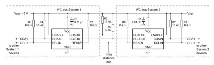
Figure 12. Repeater / Bus Extender Application Using PI6ULS5V9511B
