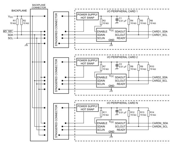
Note: The PI6ULS5V9511B can be used in any combination depending on the number of rise-time accelerators that are required by the system. Normally only one PI6ULS5V9511B is required per bus.
