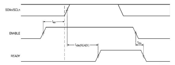
Figure 3. Timing for  $t_{\text{en}},\,t_{\text{idle}(\text{READY})}$  and  $t_{\text{dis}}$
