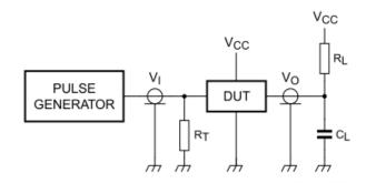
$R_L$  = load resistor; 1.35 k $\Omega$
