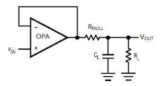
Figure 3. Capacitive Load with R<sub>NULL</sub>
