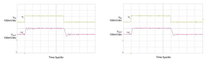
Figure 4. Test Result Without R<sub>NULL</sub>
