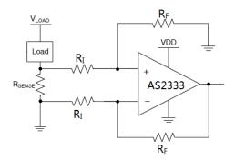
Figure 8. Low-Side Current Monitor Application
