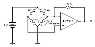
Figure 9. Bridge Circuit Amplification
