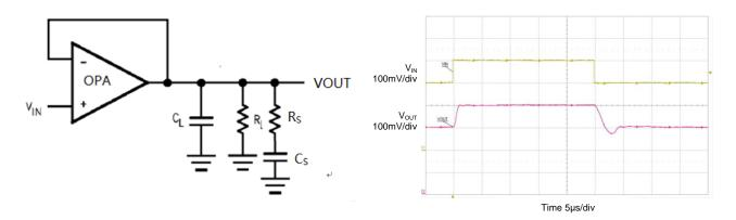
Figure 6. Circuit with Snubber Circuit
