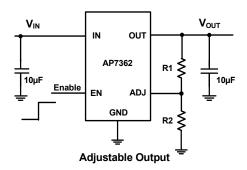
$$V_{OUT} \ = V_{REF} \left( 1 + \frac{R_1}{R_2} \right) \ \text{where} \ R_2 \leq 10 \, k\Omega$$
