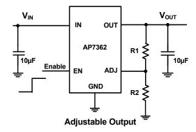
The output voltage is calculated by:
