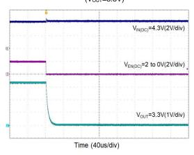
Enable Turn-Off Response (V<sub>OUT</sub>=5.0V)
