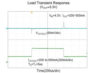
Load Transient Response (V<sub>OUT</sub>=3.3V)
