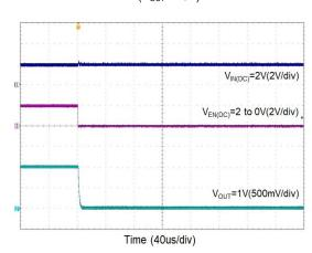
Enable Turn-Off Response (V<sub>OUT</sub>=3.3V)
