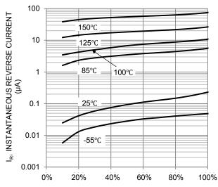
V<sub>R</sub>, PERCENTAGE RATED PEAK REVERSE VOLTAGE (%) Figure 5. Typical Reverse Characteristics
