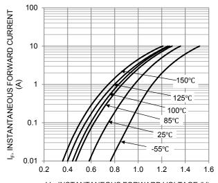
V<sub>F</sub>, INSTANTANEOUS FORWARD VOLTAGE (V) Figure 2. Typical Forward Characteristics (Per Leg)
