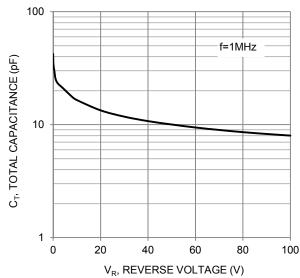
Figure 4. Typical Total Capacitance
